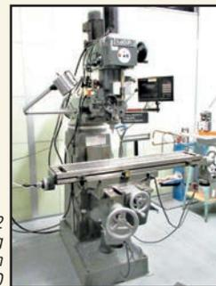
Lagun FTV-2 Vertical Milling Machine with DRO
