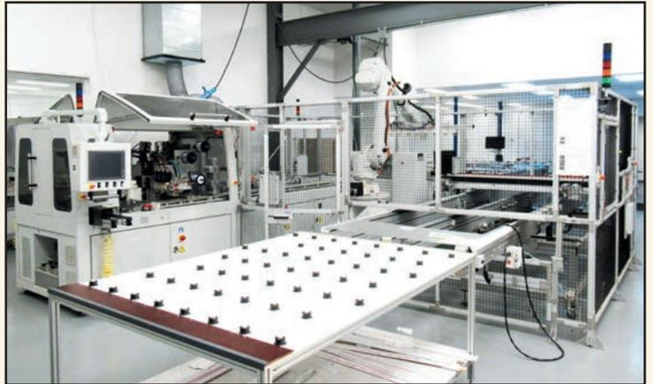
Komax Solar Automated String to Glass Lay-Up Cell
