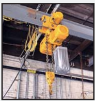
Harrington 5-Ton Electric Hoist
