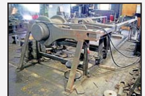
300-Ton (approximately) Horizontal Wheel Press
